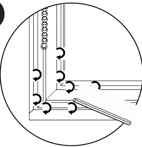
Using a tape measure or carpenter's square, ensure the frame is perfectly square, then tighten the set screws using the provided allen wrench. **DO NOT USE A DRILL OR IMPACT!** You will damage the frame.
