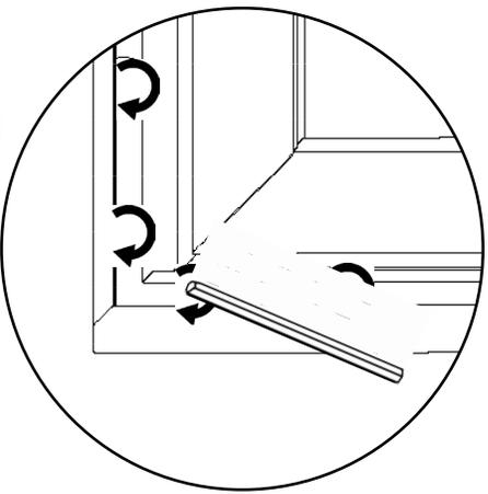
Using a tape measure or carpenter's square, ensure the frame is perfectly square, then tighten the set screws using the provided allen wrench. **DO NOT USE A DRILL OR IMPACT!** You will damage the frame.
