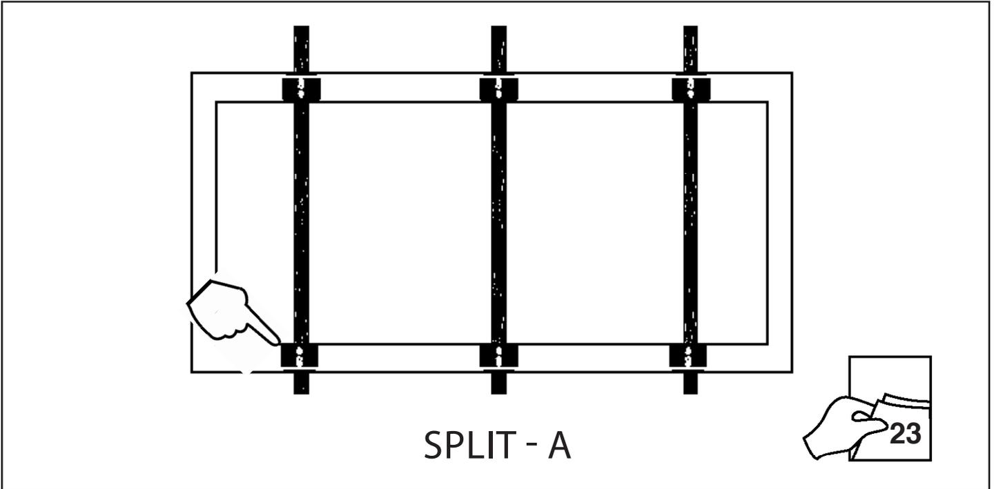
Split A mounting used when vertical support bars not being installed
