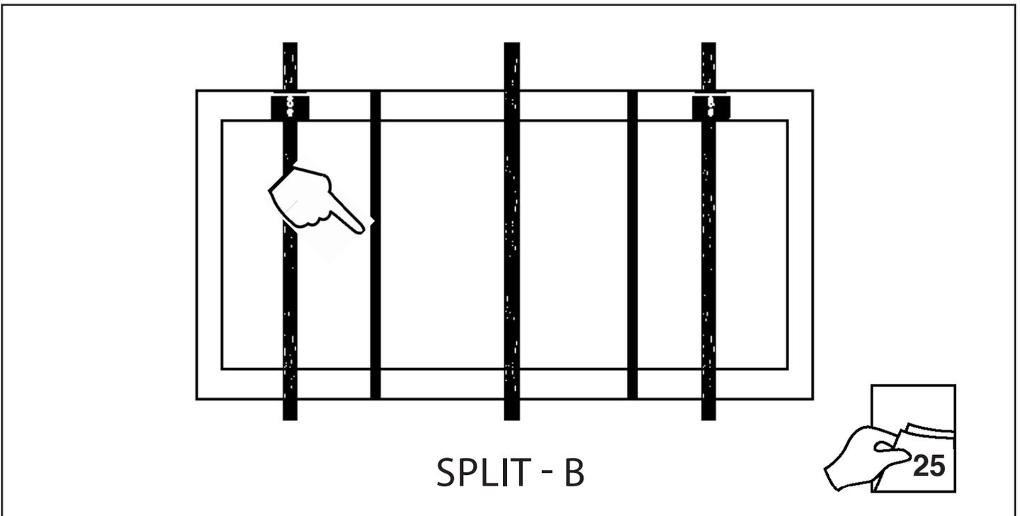
Split B mounting used when vertical support bars are installed
