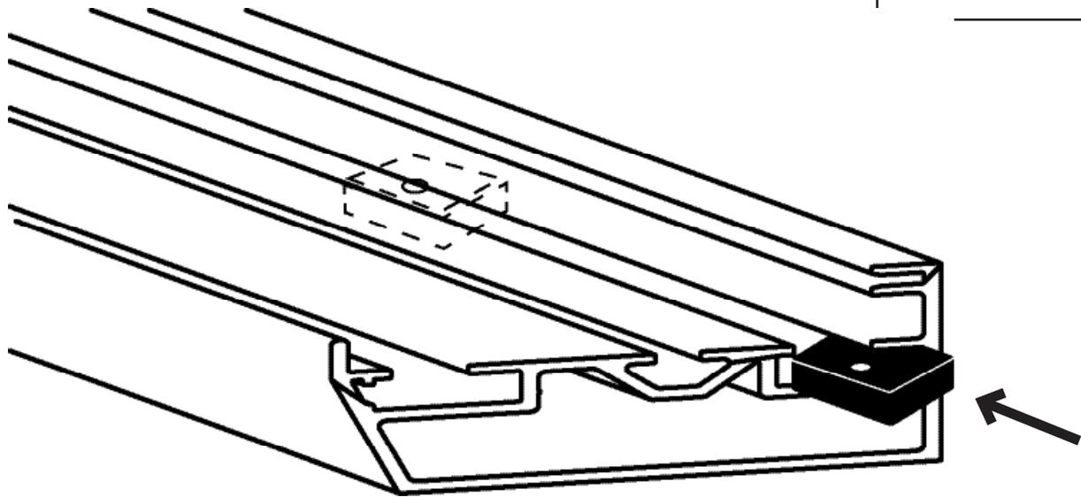
Install the t-slot nuts in the horizontal frame pieces before putting the corner brackets in.
